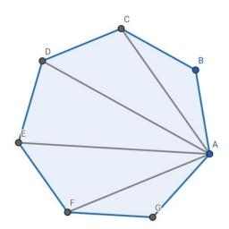
The sum of the interior angles of the polygon will be equal to the sum of the interior angles of the triangles =  $(n-2)\times180$ °
