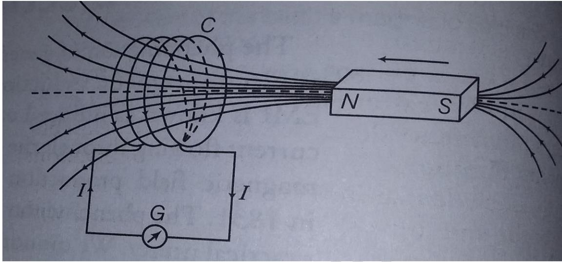
If North-pole of a bar magnet is pushed towards the coil, the pointer in the galvanometer deflects, indicating the presence of electric current in the coil. This deflection lasts as long as the bar magnet remains in motion.
