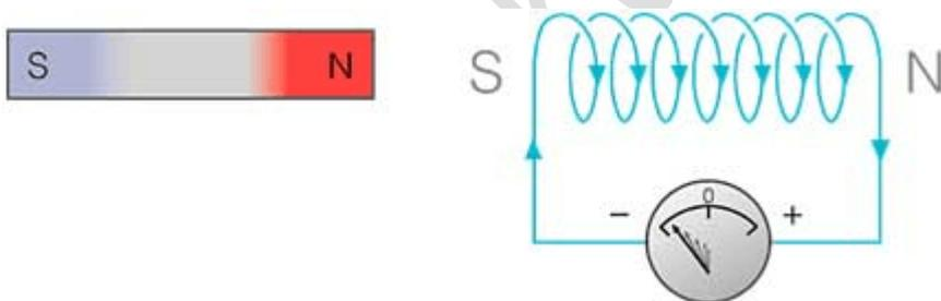
When the north pole of the magnet is moving away from the coil, the magnetic flux linking to the coil decreases. According to Faraday's law of electromagnetic induction, an EMF and hence current is induced in the coil and this current will create its own magnetic field.
