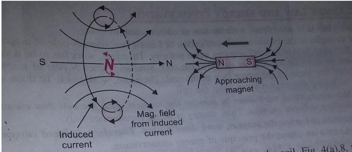
Lenz's law is based on Faraday's law of induction. Faraday's law tells us that a changing magnetic field will induce a current in a conductor. Lenz's law tells us the direction of this induced current, which opposes the initial changing magnetic field which produced it. This is signified in the formula for Faraday's law by the negative sign ('-').
