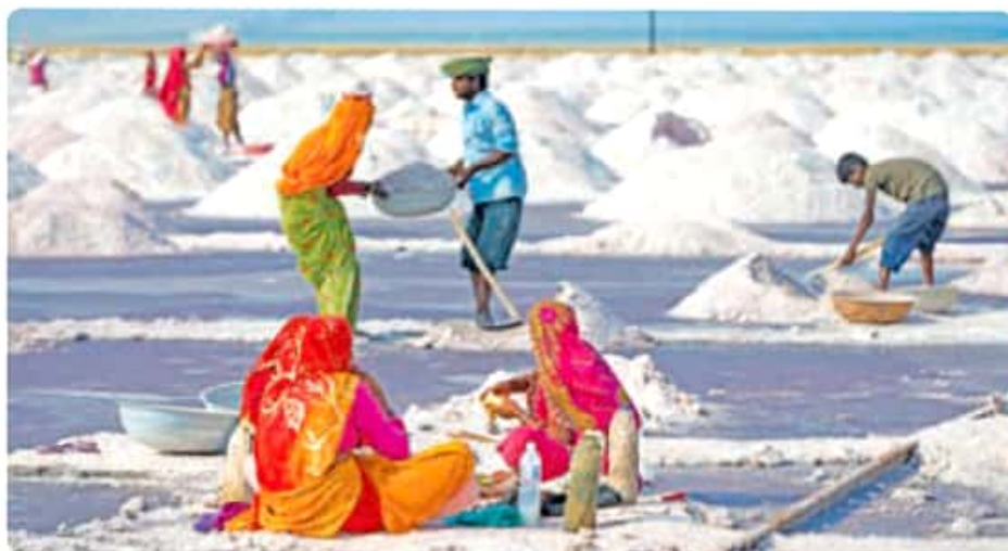
Along the coast, seawater is collected in shallow artificial ponds called salt pans. When this water evaporates, salt is left behind. This salt is then taken to the factories for refining.
